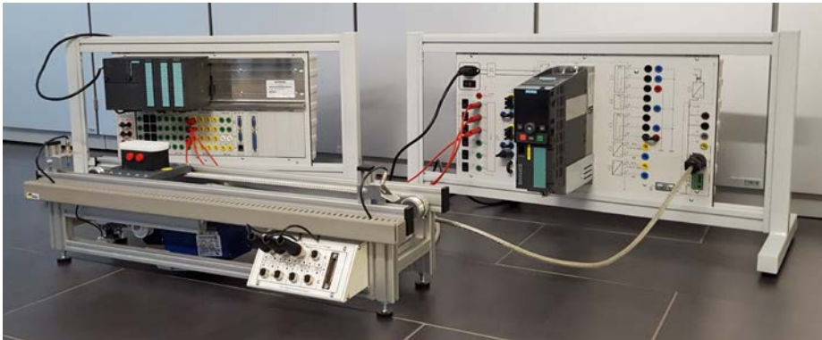
3phase AC Conveyor Belt with Frequency Converter G120 and PLC Panel
