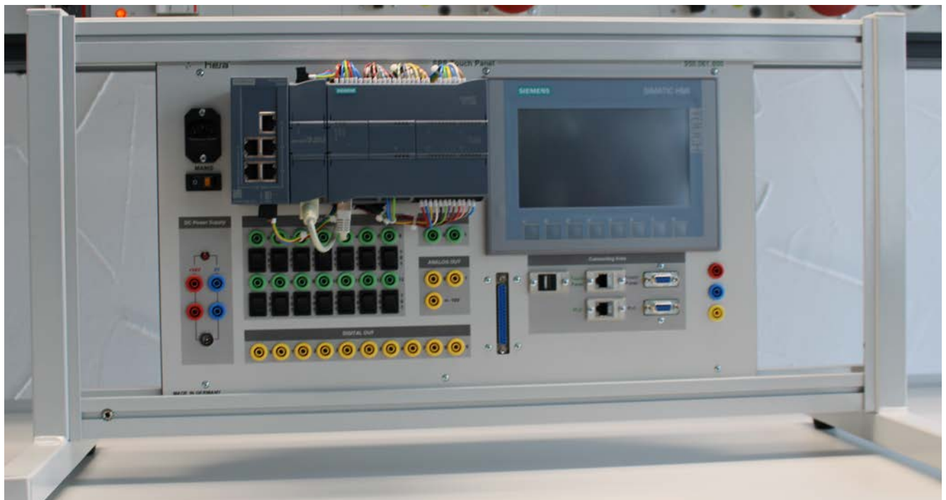
PLC Panel 950.061.600,0 with Siemens 7-1200 and KTP700 Operating Panel in Training System Frame
