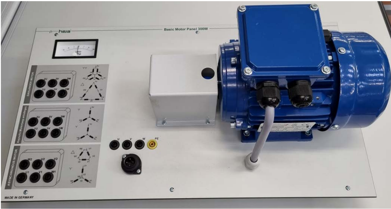
Basic Motor Panel for Control Engineering and Frequency Converter
