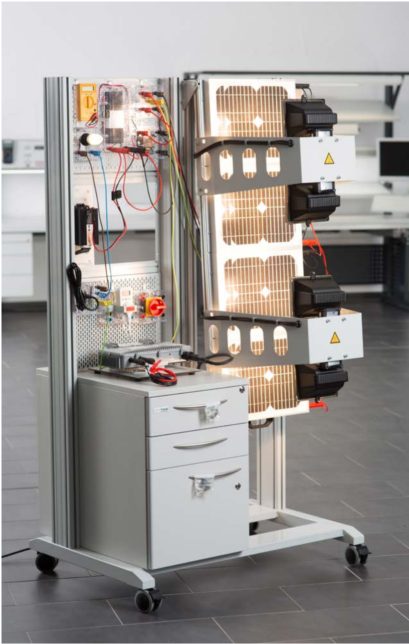
Configuration Example for Grid-Feeding and Off-Grid Technology
