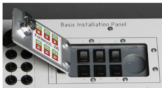
Failure Simulator with key-lock
