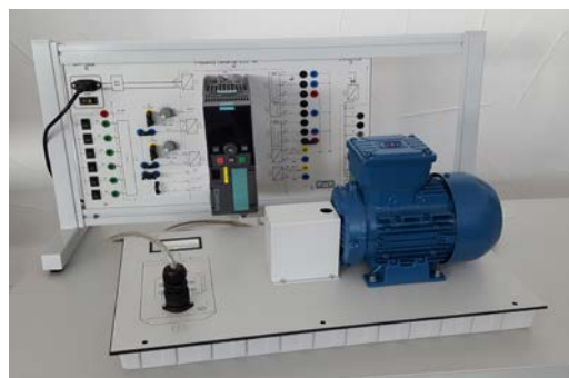
Frequency Converter with 300W Motor 540.030.630
