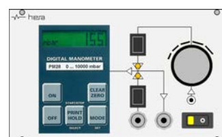
Digital Pressure Calibrator
