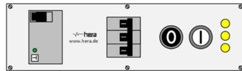
322.287.202 3phase with MCB B16, RCD type B, 2-level activation 8KP
