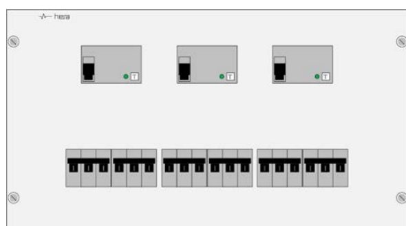
332.092.405: 19" Power Distribution for 6x 3phase with RCD (3x RCD 4poles + 6x CB B16 3phase) 6HE
