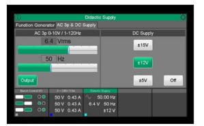
3phase Generator 1 - 120 Hz and Fixed DC Supply ±15V ±12V ±5V/1A
